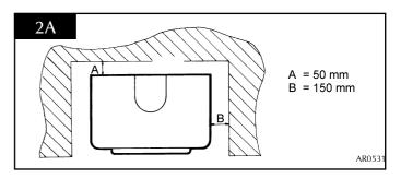
The above dimensions provide adequate clearance at the side and rear of the fire so that the controls can be reached.
